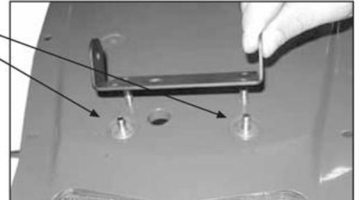
*Take away original rear fending an license plate support. Locate washers I original present flare ans insert 4 screw from the inside to the outside.
