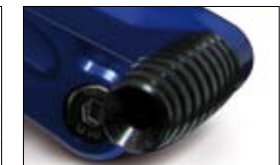
Front pegs rubber coated Puntalino rivestito in gomma
