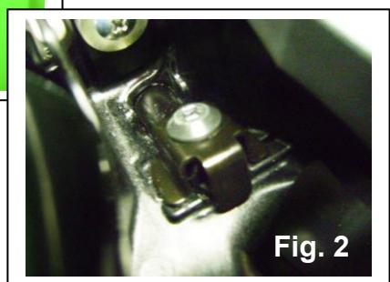
*Dismount the std. license plate holder from the rear subframe, for this operation is necessary to remove the passenger seat and disconnect the license plate light wiring ( Pic 1 )*
