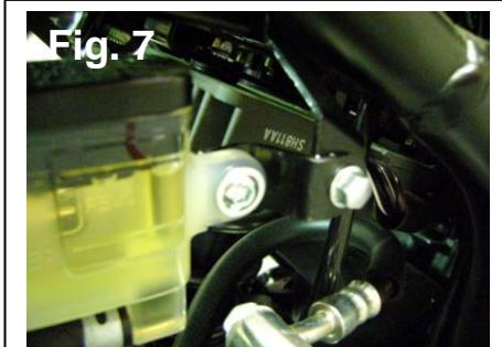
*Remove the brake fluid reservoir tank from its place using the dedicated bracket (pic. 7).*
