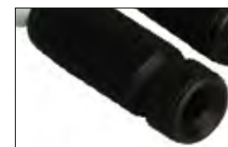
Footpegs with special shape "no slide", to increase the contact with the boot
