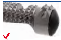
CNC machined nylon caps protectors at the end of footpegs
